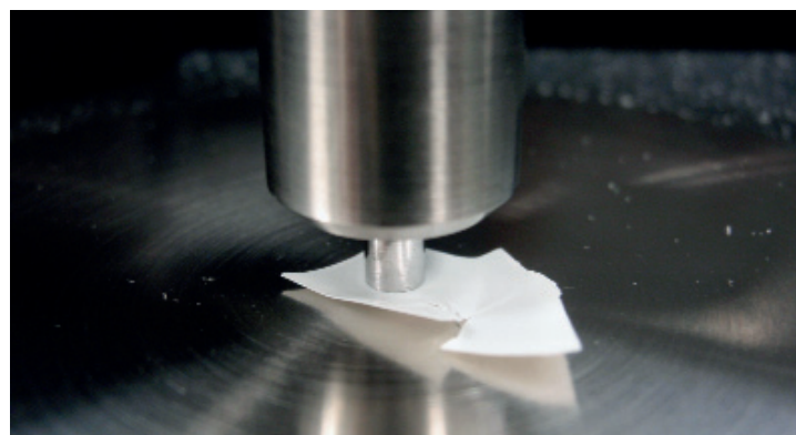
Figure 1: The pressure rod of the DuraSAMPLIR pushes a disintegrated piece of the plastic bag against the diamond prism
