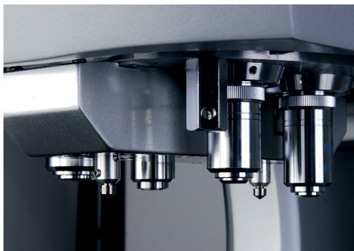
Figure 2: Multi turret function with up to two indenters and four objective lenses
