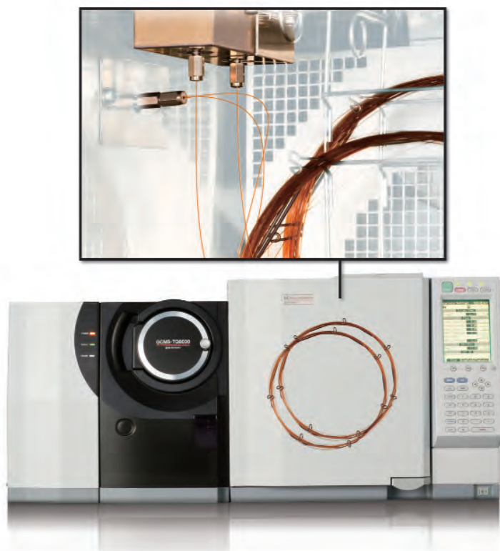
Figure 4: Twin-line configuration of the GCMS-TQ8030
