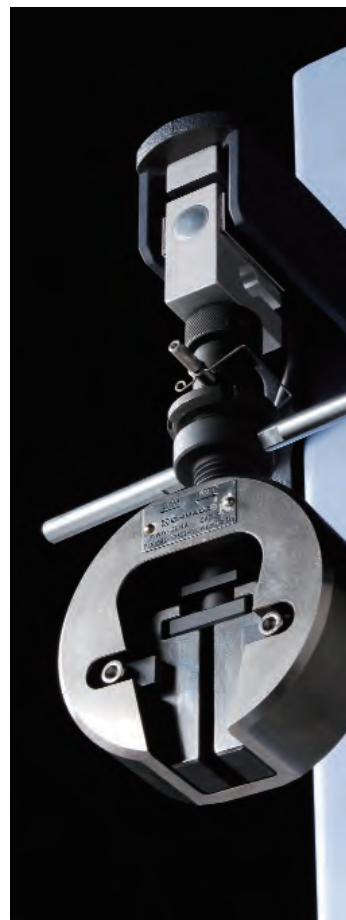
Figure 2: Modern non-shift wedge type grips in combination with a high-precision load cell
