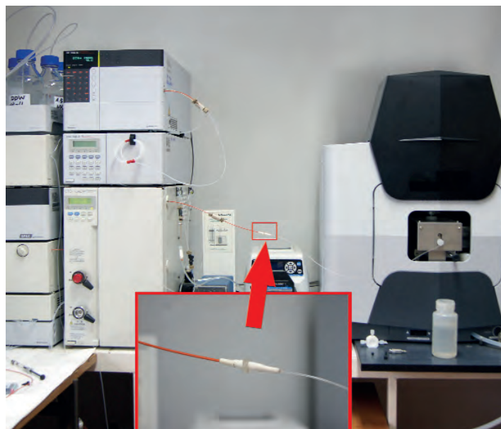
Figure 1: The HPLC-FAAS analytical system used in the laboratory of Department of Water and Soil Analysis, Faculty of Chemistry, Adam Mickiewicz University, Poznań, Poland
