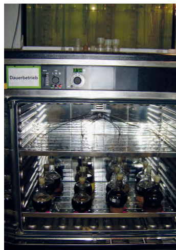
Figure 1: Experimental setup for biogas production in the laboratory
