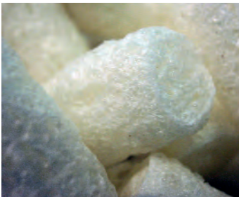
Figure 1: Edible packaging material: a packaging chip made out of starch
