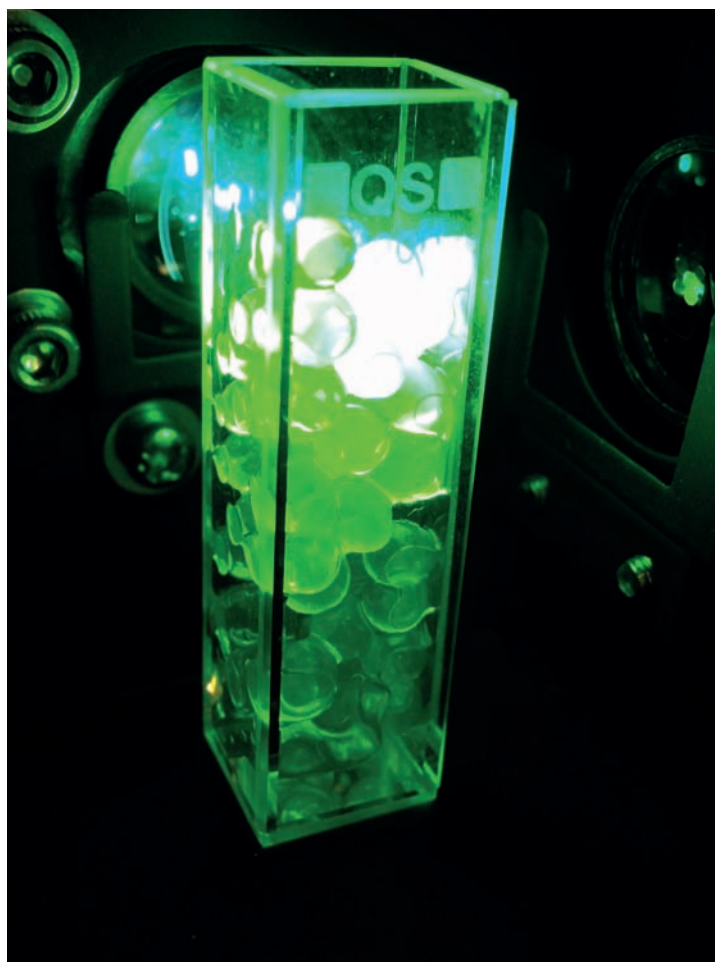
Figure 1: Alginate based Caviar prepared with fluoresceine excited with analytical wavelength of 460 nm in a Shimadzu fluorescence spectrophotometer RF-5301PC: it is fluorescent caviar filled into a 1 cm quartz cell
